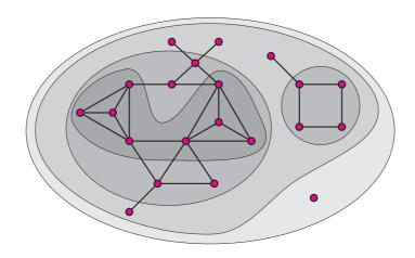
Cores can be computed according to lines going into vertices (Input), lines going out of vertices (Output) or all lines (All). In the case of undirected networks input and output cores are the same.
