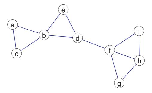
Te network in the picture (<u>aho1.net</u>) consists of 4 biconnected components:
