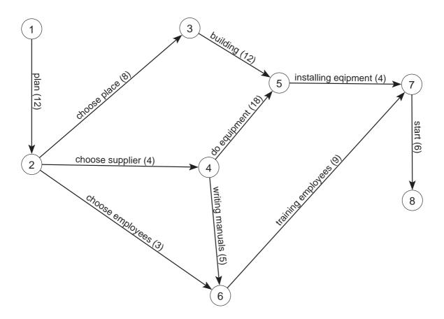
In a CPM network we want to find a critical path which determines the time needed to finish the whole project. In our example the critical path is 1 - 2 - 4 - 5 - 7 - 8, and the duration is 44.
